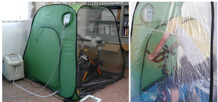
Fig. 1 Normobaric–intermittent hypoxic tent equipped for research [143] and used to trained climbers for an Everest expedition, 2011 (unpublished results)
